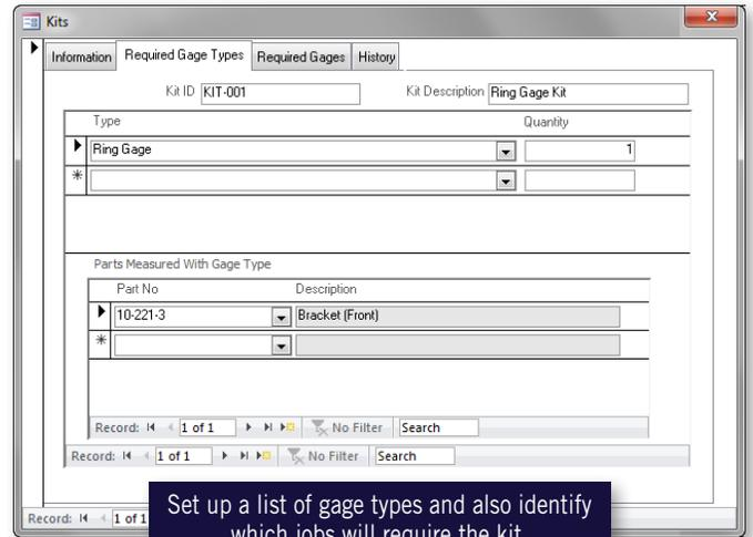
Set up a list of gage types and also identify which jobs will require the kit.
