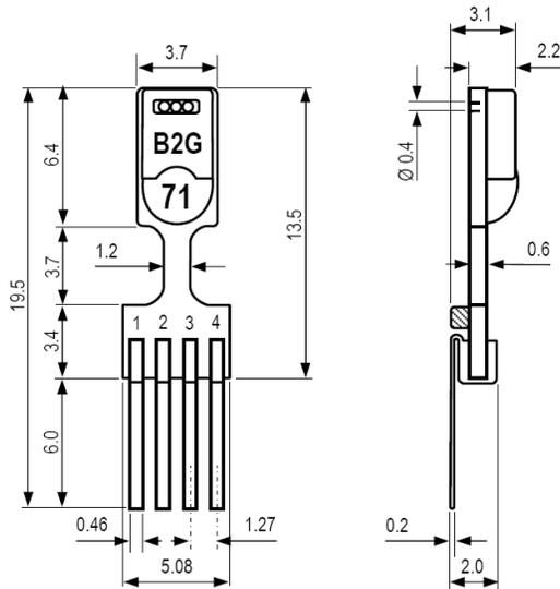
**Figure 1:** Drawing of SHT7x (applies to SHT71 and SHT75) sensor packaging, dimensions in mm (1mm = 0.039inch). Contact assignment: 1: SCK, 2: VDD, 3: GND, 4: DATA. Hatched item on backside of PCB is a 100nF capacitor – see Section 2.1 for more information.
