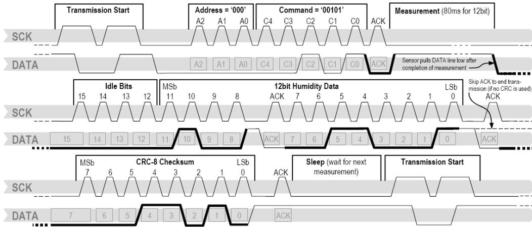
**Figure 12:** Example RH measurement sequence for value "0000'0100'0011'0001" = 1073 = 35.50%RH (without temperature compensation). DATA valid times are given and referenced in boxes on DATA line. Bold DATA lines are controlled by sensor while plain lines are controlled by the micro-controller.
