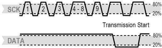
Figure 8: Connection Reset Sequence
