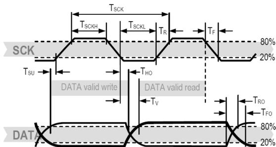
**Figure 6:** Timing Diagram, abbreviations are explained in Table 3. Bold DATA line is controlled by the sensor, plain DATA line is controlled by the micro-controller. Note that DATA valid read time is triggered by falling edge of anterior toggle.
