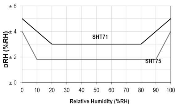
Figure 2: Maximal RH-tolerance at 25°C per sensor type.
