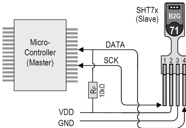
**Figure 5:** Typical application circuit, including pull up resistor R<sub>P</sub>.
